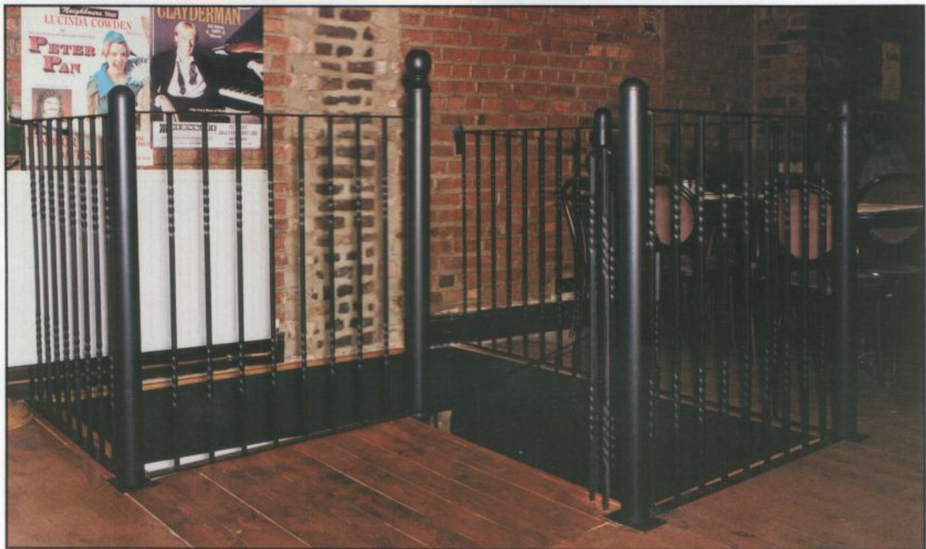
Fig. 3. Features the E8 Double Twist Baluster. The picture also shows how Elite has used the E8 Baluster to complete the Guard Rail around the opening. The rail is 1100mm high to comply to Building Regulations BS5395 Part K, 1984.
